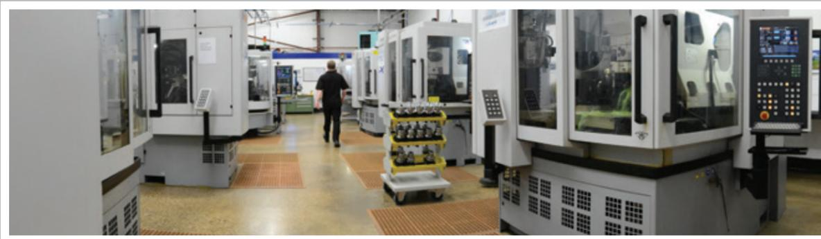
Heavy investment in cutting edge machinery facilitates rapid tool production. A thermally controlled atmosphere maintains quality and repeatability.
